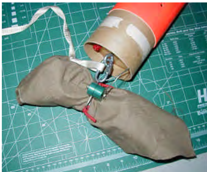
Figure 4 – The completed assembly is then securely attached to the payload bay eyebolt with a carabineer through one of the large holes in the metal tab. The e-match wires are not shown in this photo. They would be attached to the two red screw-terminals. Note that only a short length of ematch cable is required.
