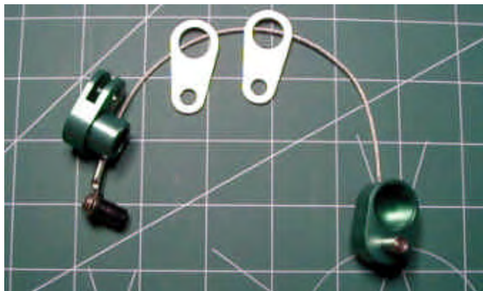
Figure 1 – These are the basic pieces of the Tether. The grid squares are one inch on a side. The rubber stopper seals the charge compartment in one half of the locking mechanism. The wire harness for the e-match exits the charge compartment alongside the rubber stopper. The steel cable is run through one of the tabs and keeps both halves of the locking mechanism from being lost.
