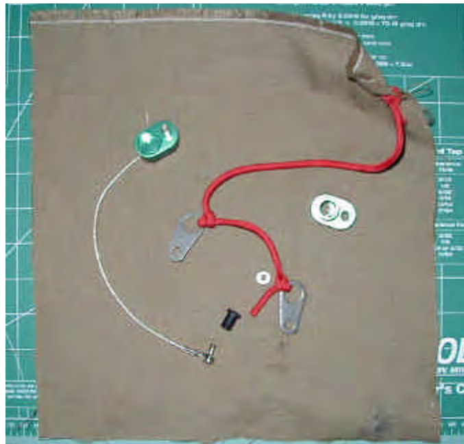
Figure 2 – The user supplies a piece of cloth (a Pratt Hobbies Nomex parachute protector in this case) to wrap the parachute and shock cord. The red parachute cord and the two metal tabs hold the parachute inside the cloth until the locking mechanism releases.
