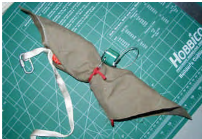
Figure 3 – The parachute is securely wrapped inside the cloth and held in place by the parachute cord and tabs. The green locking mechanism is then held together with a small piece of masking tape. The tape will yield when the pyrotechnic charge is initiated and the locking mechanism will fly apart.
