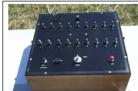
A closer view of the new controller shows the 18 LED toggle switches; the black continuity check button to the lower left; piezo beeper; arming circuit at the center; and the red firing button on the right.
