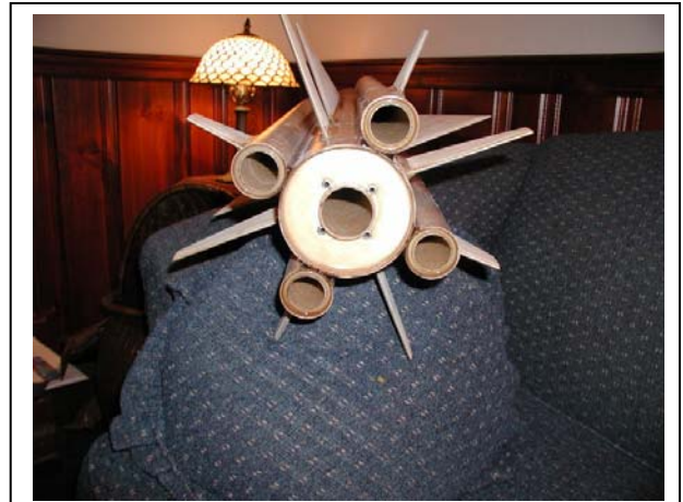
Rear of the SA-5 Gammon showing igniter conduits and heavy fillets for the outboard motor tubes.
