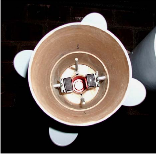
Completed avionics bay showing mounted timers, plugged forward closure of centerline motor, igniter conduits, and threaded rods for securing bulkhead.
